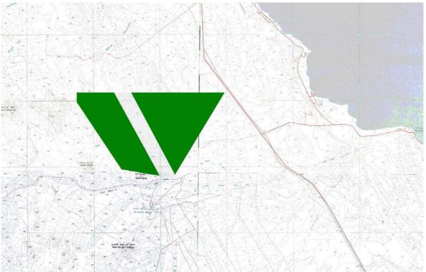
Figure VIII.1: Schematic illustration of an "escape corridor" within a huge wind farm. Note that the corridor is orientated parallel to the dominating wind-direction.
