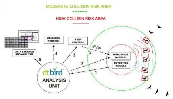
Figure VIII.2: Schematic illustration of a detection and dissuasion system.
