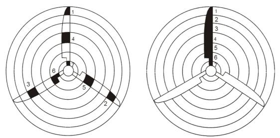
Figure VIII.2: Proposed patterns of painting turbine blades (according to Hobos 2003): a black bar on one blade is not repeated in the same location on the other two blades (left); a single-blade, anti-motion-smear pattern (right).
